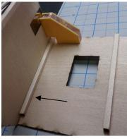
I use these magnet corner clamps to help keep it square and tape the outside corners to hold it in place as the glue sets up. Glue the inside corners and add the 3½" X 1/8" X 1/8" braces. Make them flush with the bottom too.
